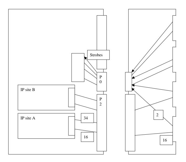
Notice how 16 actual I/O lines and 34 'spares' connect each IP site and the transition card connectors and how two strobe lines from each connector are collected at P0 and brought through along with the site D signals.
