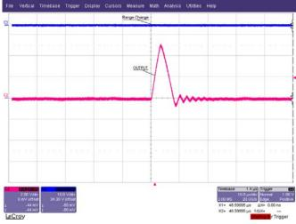
When going from +/-5V to 0-10V then only first glitch to 2.5V. When going from 0-10V to +/-5V only second glitch at 2.5V.
